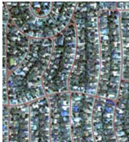
Figure 2 Road centerlines are extracted from QuickBird data in two steps: first by getting a polygon rendering, then converting the polygon to a centerline.
